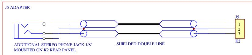
**Additional, fixed level audio output cable adapter from K2 - J5**
