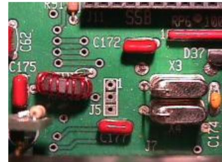
Additional, fixed level audio output cable adapter from K2 - J5
