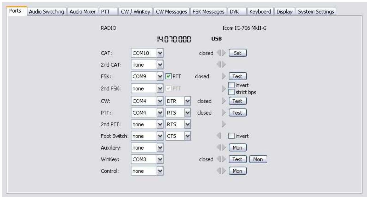
4. On the **PTT tab** select **PTT1** for VOICE, **PTT1 or QSK** for CW and **PTT2** for FSK/DIGITAL. Check PA PTT if microKEYER will be controlling an amplifier PTT line.
