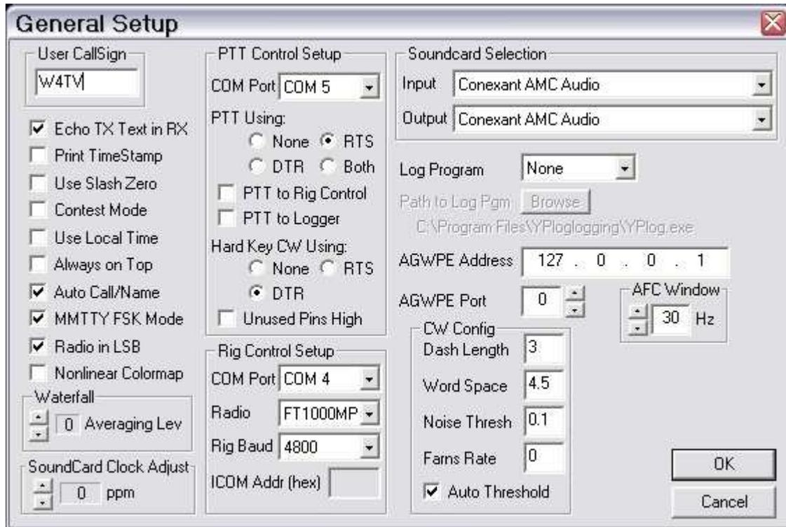
2. If you intend to use FSK with MMTTY check the "MMTTY FSK Mode"
